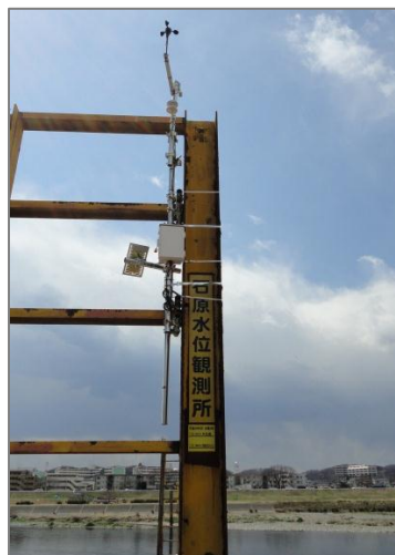
Figure 4.6 Meteorological station installed at S6, recording solar radiation, air temperature, relative humidity and wind velocity.
