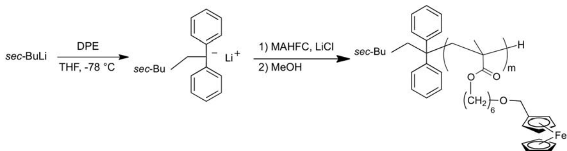
Figure 3-3-3. Synthesis of PMAHFC homopolymer by living anionic polymerization.
