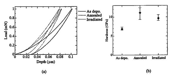
Fig. 5 Nanoindentation (a) load-depth curves and (b) hardness of as-deposited, annealed and irradiated films
