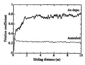
Fig. 3 Friction coefficients of as-deposited and annealed film
