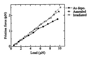
Fig. 4 Friction coefficients of as-deposited, annealed and irradiated film measured with SPM
