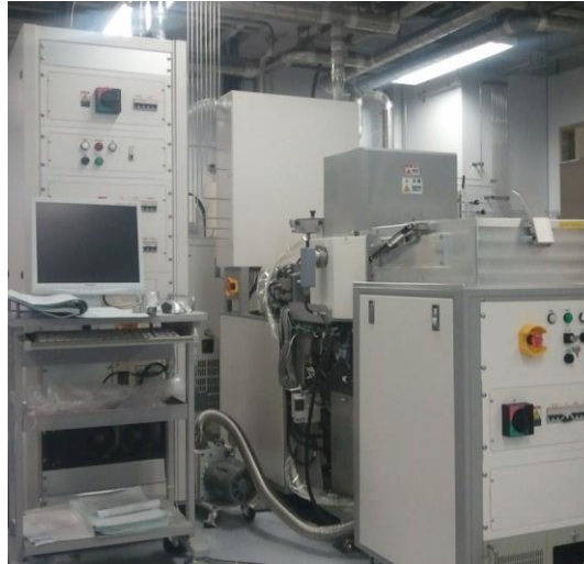
Figure 2. 5 PECVD equipment for a-Si:H deposition
