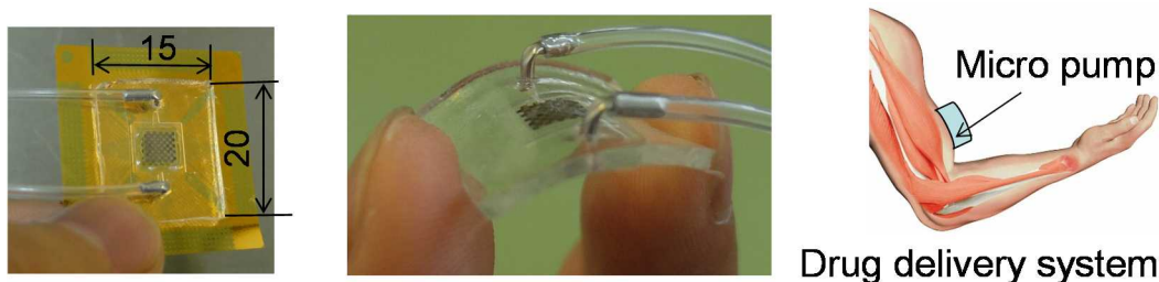
Fig. 1.4 Flexible micro pump prospective view and its future application
