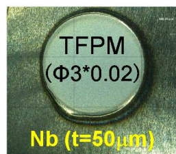
Fig. 2.10 Sputtered 20μm thick TFPM on 50μm thick Nb substrate
