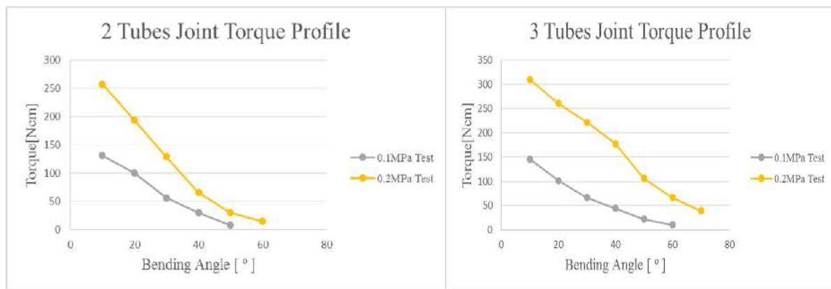
Figure 15: Test result for flat tube with hinge joint
