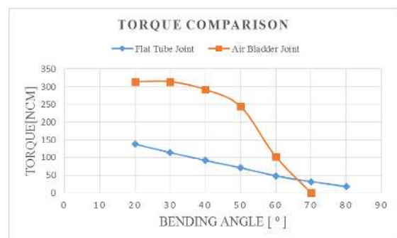
Figure 17: Torque comparison graph
