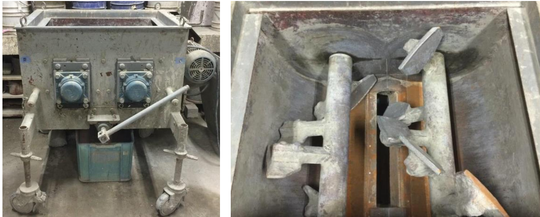
Photo 3.2.2 Biaxial mixer for mixing PP-ECC.
