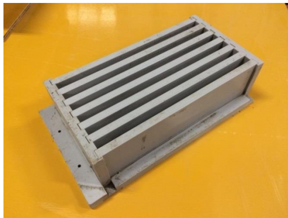
Photo 3.4.1 Formwork for uniaxial tensile tests.
