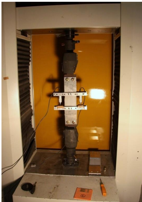
Photo 3.4.2 Experimental setup of the uniaxial loading tests.
