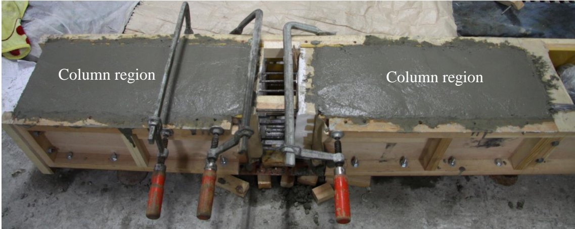
(a) Casting concrete in column regions.
