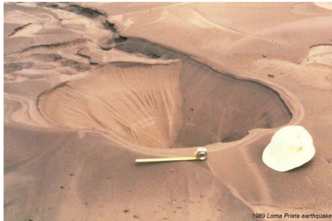
Figure 1.1. Sand boils during 1989 Loma Prieta earthquake (University of Washington, 2000).
