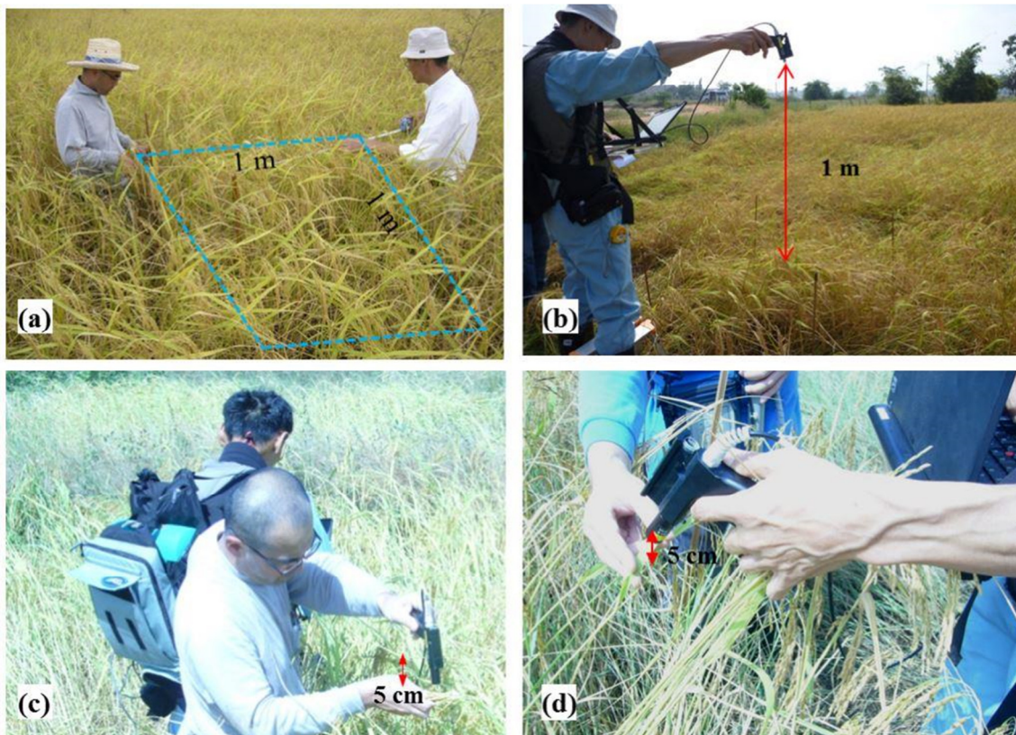
Figure 3.3 Reflectance measurement procedures: (a) quadrat 1 m × 1 m, (b) canopy reflectance, (c) grain reflectance, and (d) leaf reflectance
