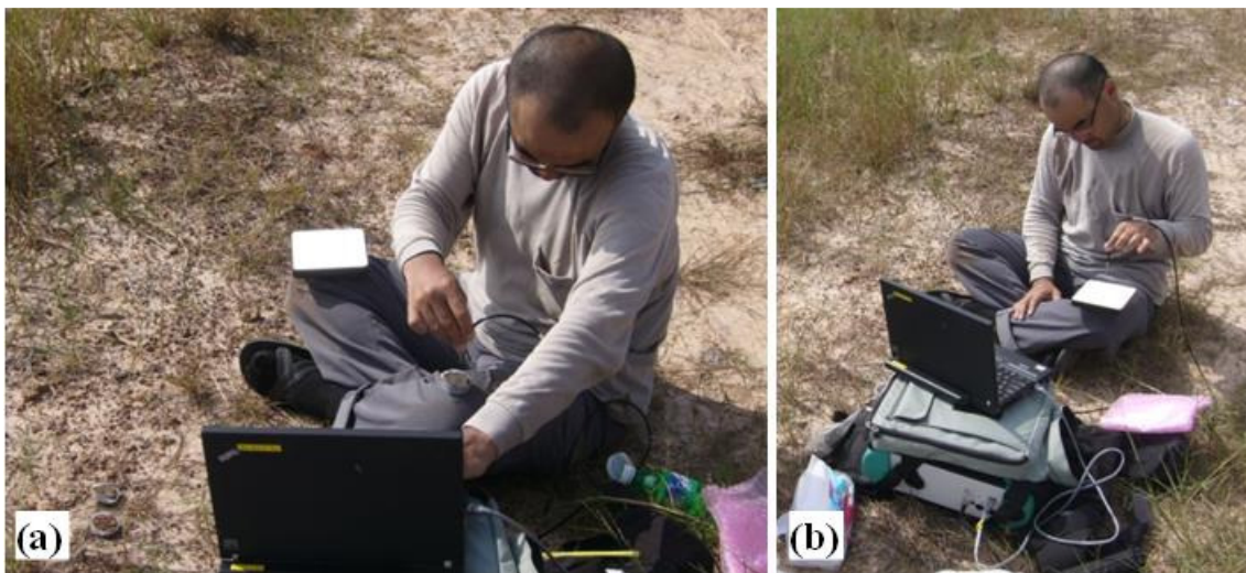
Figure 4.5 Field measurement: (a) soil reflectance measurement, and (b) calibration with ceramic pad.
