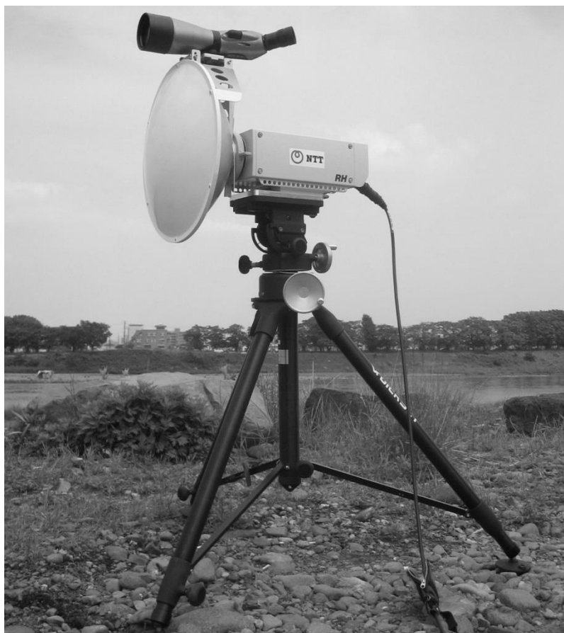
Figure 1-2. Outward appearance of 120-GHz band wireless transmitter
