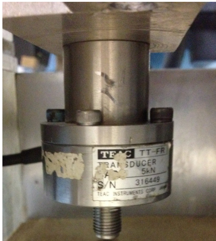
Figure 3.29 Load cell for pile load test
