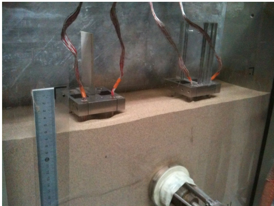
Figure 3.48 Complete preparation of model ground with pile groups
