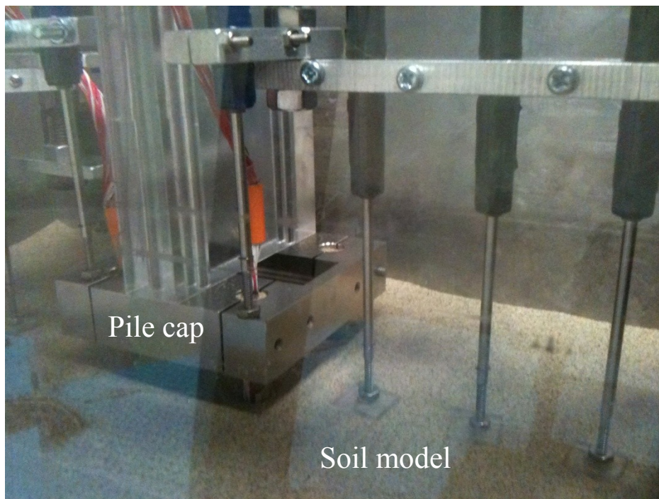
Figure 3.27 PTM on the pile cap and on the soil model
