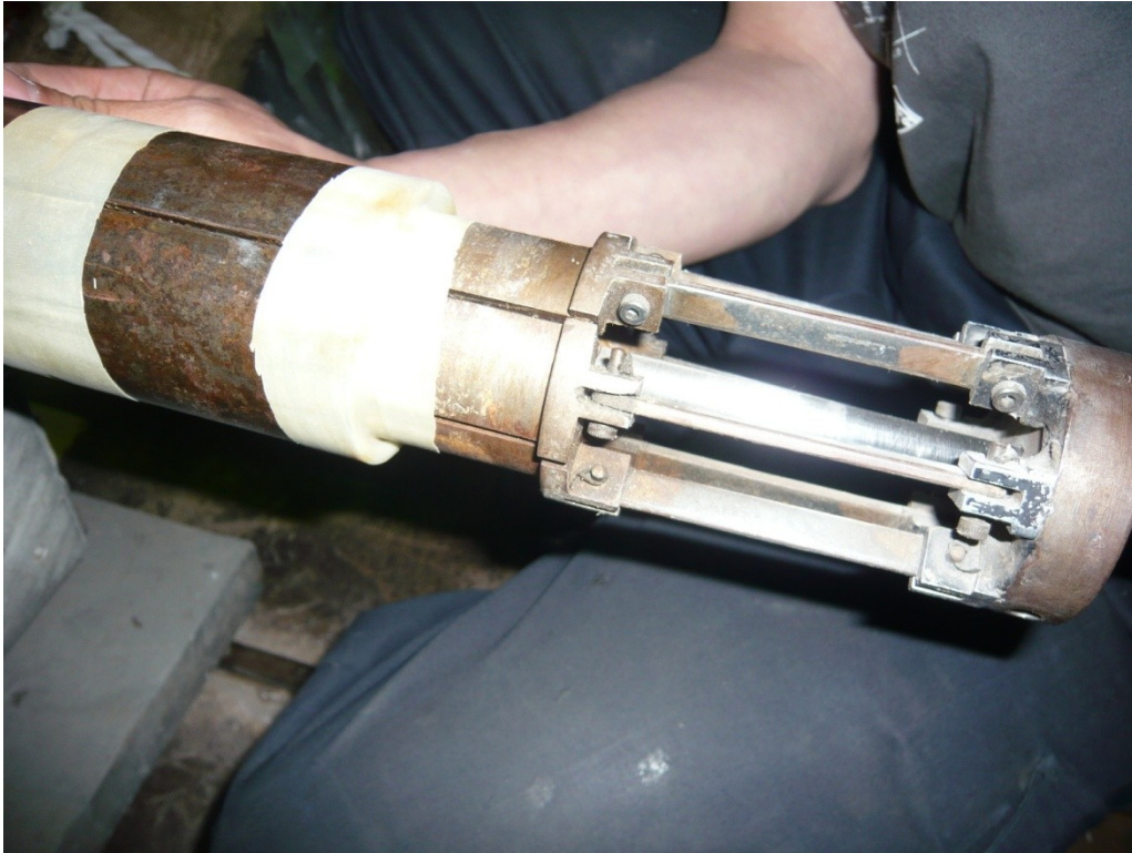
Figure 3.6 Divided steel rings and wedge-shaped shaft of tunnel machine
