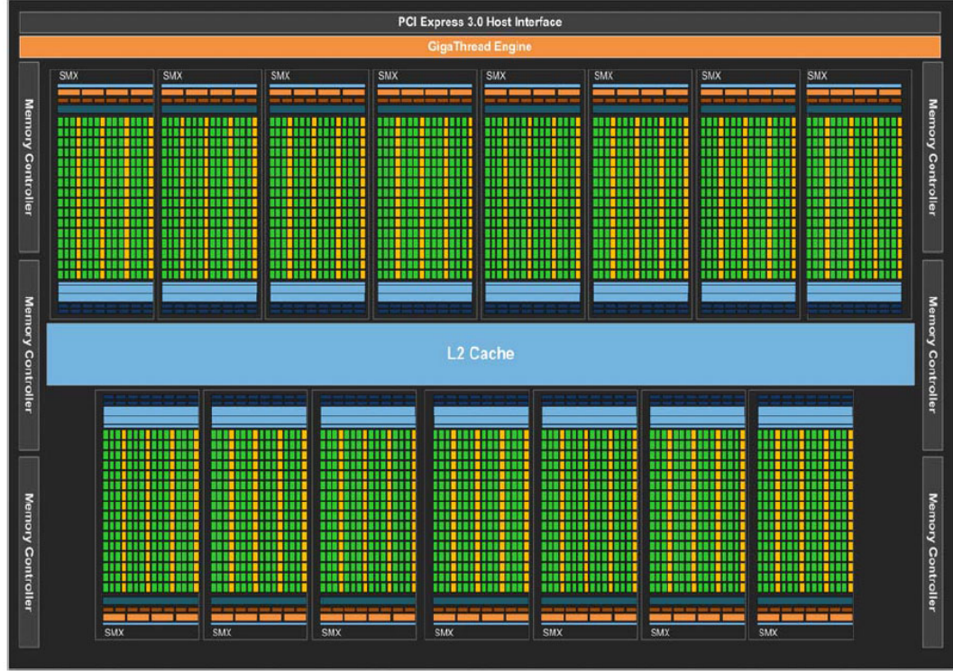
FIGURE 2.3: Kepler architecture. Source: NVIDIA Corporation (2012) [2]
