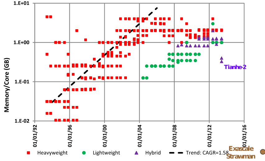
Figure II.1: Evolution of the memory capacity per core for the machines on the Top500 list, by Kogge et al. [49]
