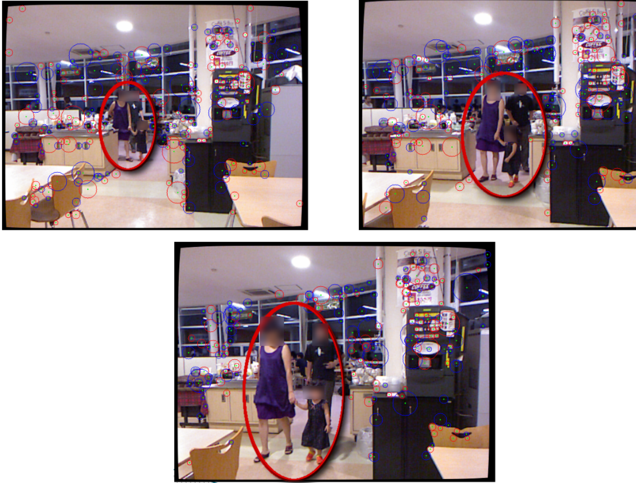
FIGURE 6.4: Appearance of double-directional ICGM's extraction. Pedestrians within red circles were walking. Small blue circles are feature points which centers are darker than backgrounds. Small red circles are opposite. Red feature points' centers are brighter than backgrounds. Each circle's radius is refers to detected scale of each feature point.
