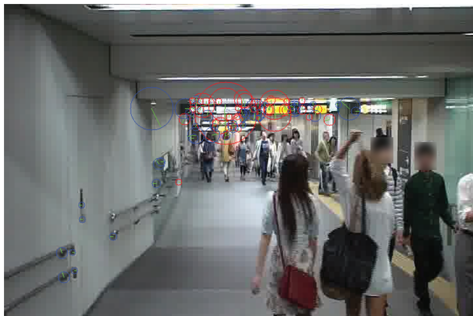
(c) Visual-feature extraction's result on the basis of Experiment B. normalize circles with different colors represent extracted visual-features. Dynamic components of this environment are ignored correctly.
