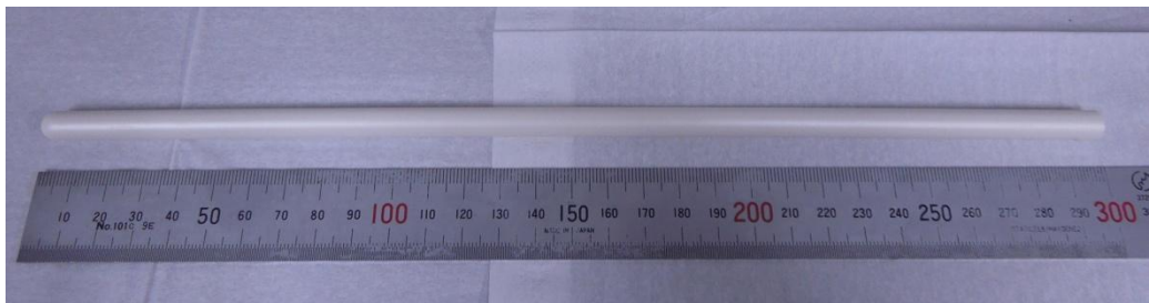
Fig. 3.5 Tubular YSZ electrolyte.
