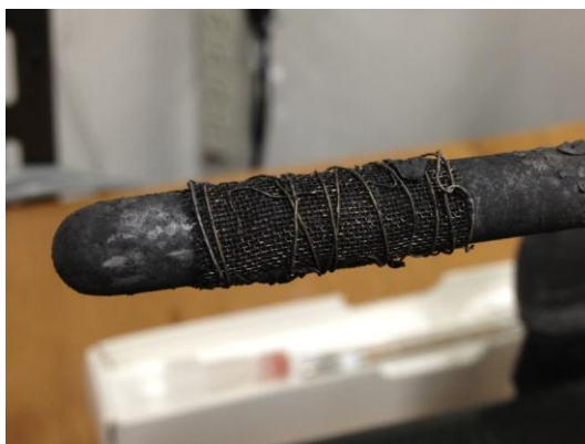
Fig. 4.10 Ni-LSM|YSZ|LSM-YSZ cell after tested over 600 h.
