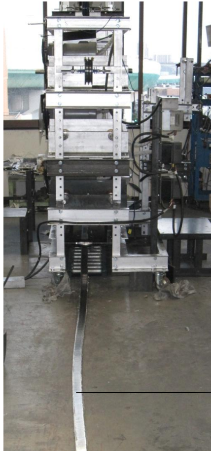
Fig. 2-14 Outlook of three-layered clad strip fabricated by using the vertical-type high-speed tandem twin-roll caster.
