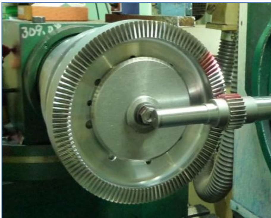
Fig. 5.25 Meshing test of face gear
