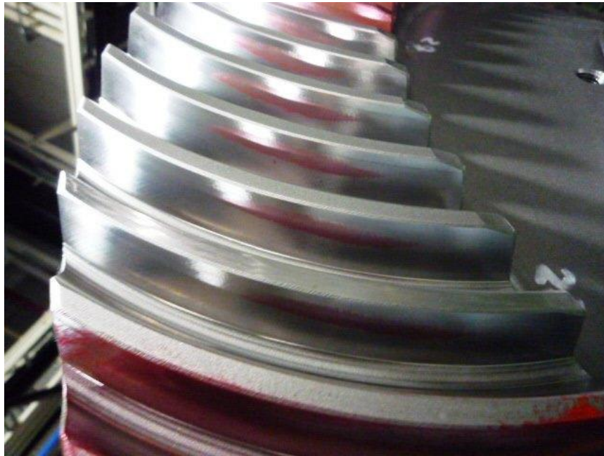
Fig. 3.20 Result of meshing test for gear drive side
