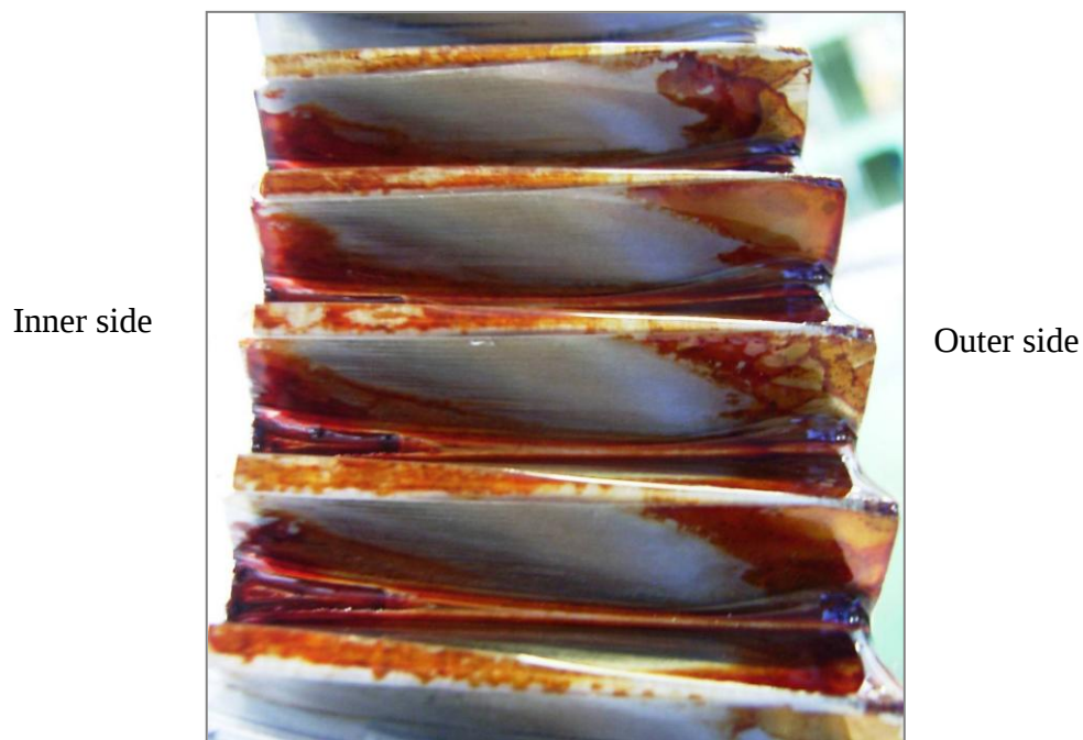
Fig. 5.29 Tooth contact patterns after running test
