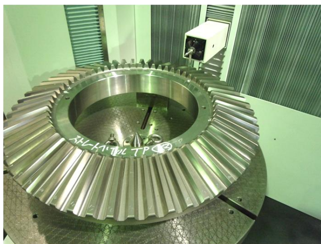
Fig. 5.8 Measurement of gear member
