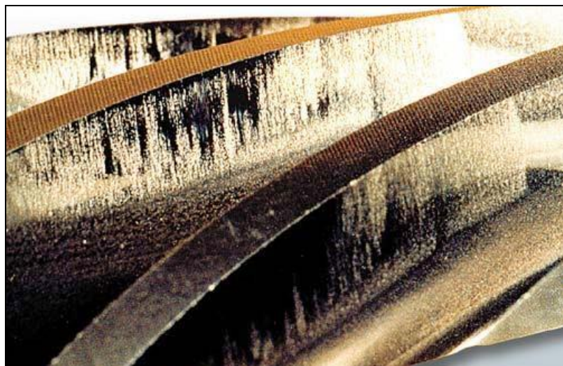
Fig. 3.1 Scuffing damage at addendum of pinion tooth surface
