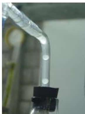
Fig. 5.12 Adjusting the flow by counting the oil drops
