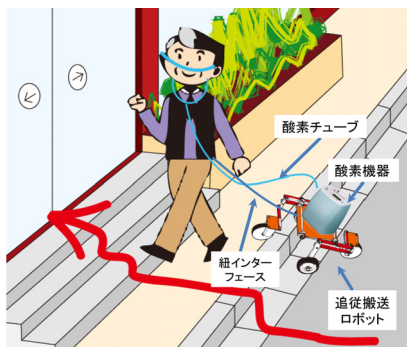
Fig.1 Basic concept of the robotic follower carrying an oxygen equipment
