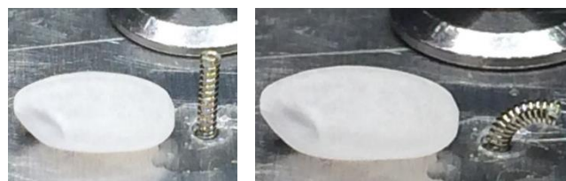
Fig.9 Model 2 which can be bend in all directions (outer diameter:0.60mm)
