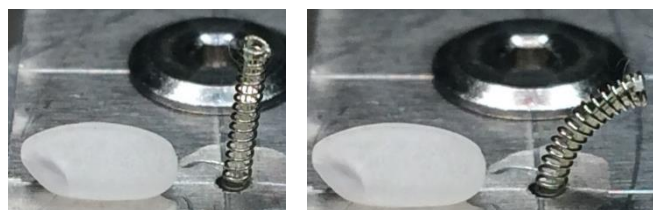
Fig.8 Model 1 which can be bend in all directions (outer diameter:0.92mm)
