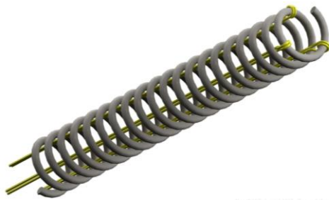
Fig.2 Magnified figure of the tip bending mechanism
