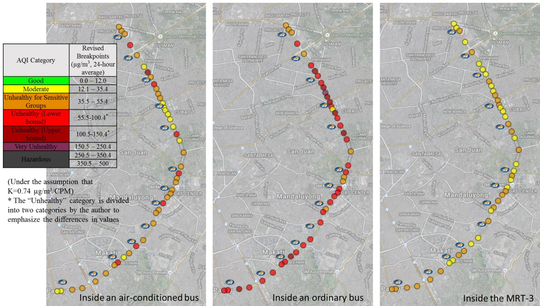
Figure 4.10. Comparison of measured particle count averages between the interiors of the MRT-3, air-conditioned bus, and ordinary bus
