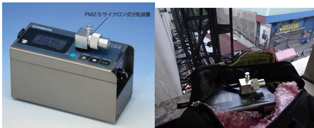
Figure 4.1. SIBATA PM 2.5 Cyclone for LD-5 equipment
