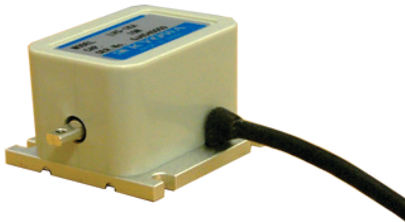
Photograph 5-1 Miniature load cell (Kyowa Electronic Instruments Co., Ltd., LVS-2KA) (Reference Kyowa Electronic Instruments Web site)
