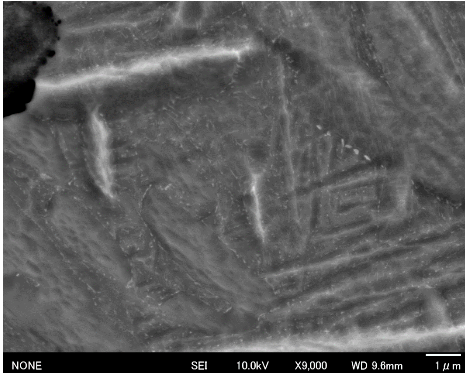
Figure 4. 10 High magnification SEM image of sintered at 700 °C, 30 MPa sample solution treated at 1000 °C for 1 hour then aged at 530 °C for 6 hours
