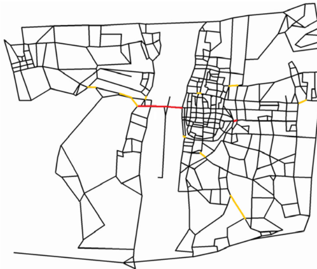
(b) The congestion distribution under 1500 Floyd agents and 1500 Adaptive agents on a real road map
