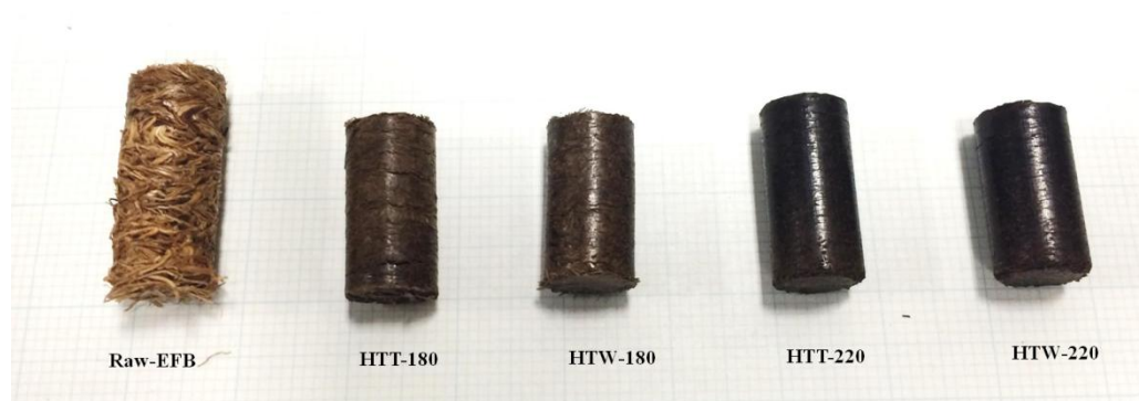
Figure 4-5. The appearance of the pellets made from raw-EFB, hydrochars and washed hydrochars
