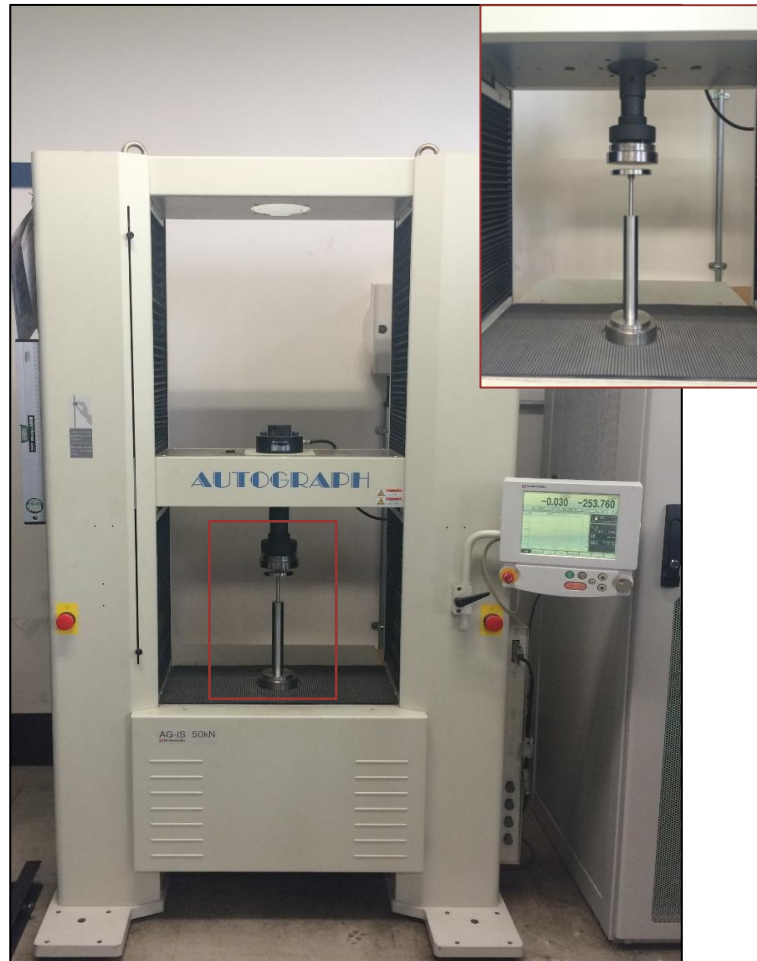
Figure 4-1. The pelletization unit set up
