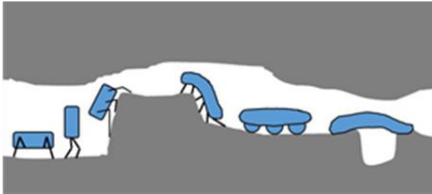
Figure 5-5 Concept image of running in rough terrain with transformable mobile robot.
