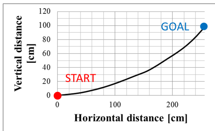
Figure 6-10 Slope shape in target terrain
