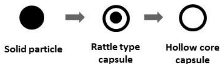
Figure 1.11 The hollow core capsule formation process by Ostwald ripening method
