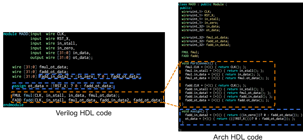
Figure 5.3 The correspondence relationship between Verilog HDL and ArchHDL
