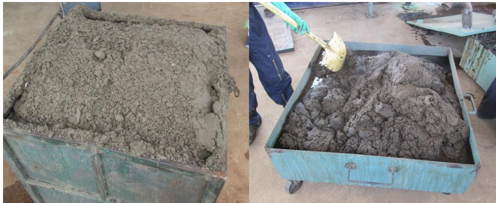
Figure 2-8 Paper sludge before (left) and after hydrothermal treatment (right)
