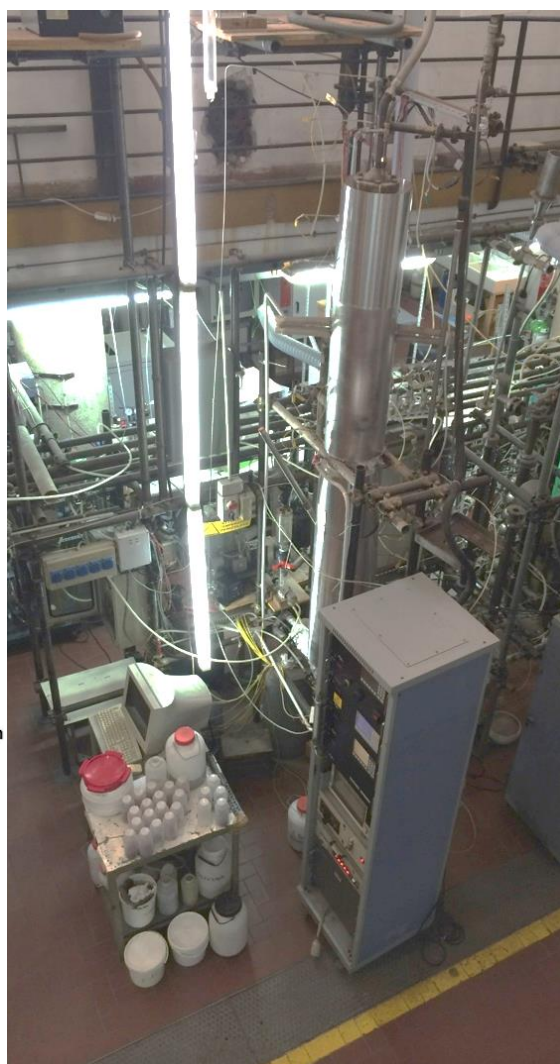
Figure 5-1 The 110 mm ID stainless steel fluidized bed combustor
