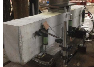
Fig. 31 Geometry of the RC beams (left) and measurement devices installed on the beam (right).
