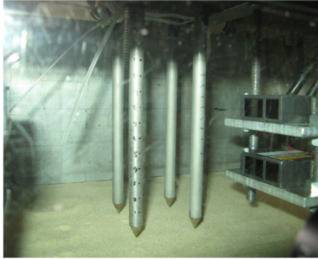
Figure 3.5.2 Model foundation fixed to actuator using guide rods for (a) piled raft and pile group, (b)raft.
