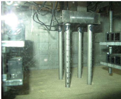
Figure 3.5.3 Penetrated piles by deadweight in gravitational field.
