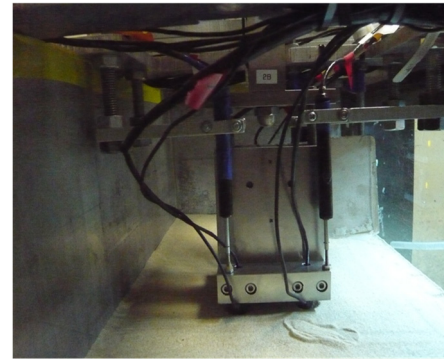
Figure 3.5.5 Model piled raft and pile group after setting instrumentations.
