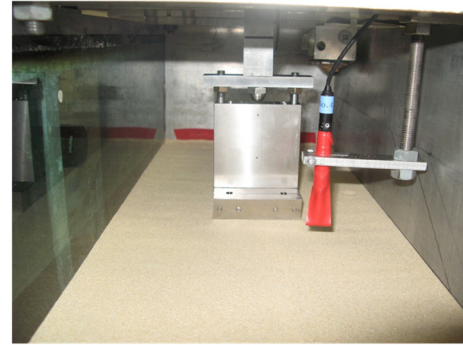
Figure 3.5.2 Model foundation fixed to actuator using guide rods for (a) piled raft and pile group, (b)raft.
