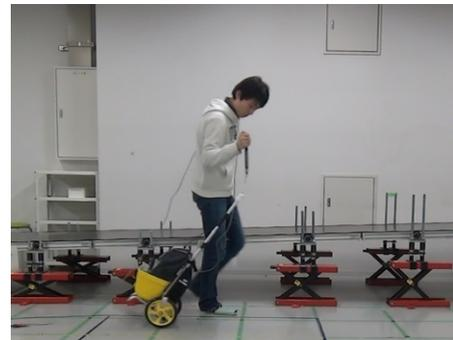
Fig.14 Towing experiment: the participant towed the prototype robotic cart by applying the spring scale to measure the holding force.
