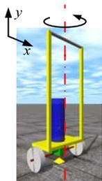
Fig.7 Inverted pendulum control evaluation; After adding the twist torque at 0.5s for the Y axis, behaviors of the robotic cart are observed.
