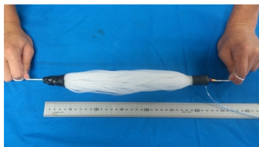
Fig.2 Multifilament pneumatic muscle (Air pressure 0.25MPa)
