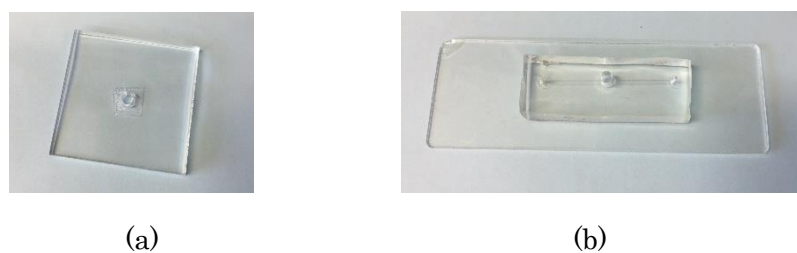
Figure 2.13. Photos of the chambers. (a) Static chamber. (b) Flow chamber.
