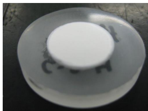
Fig.3-17 樹脂包埋、鏡面研磨後の試料
