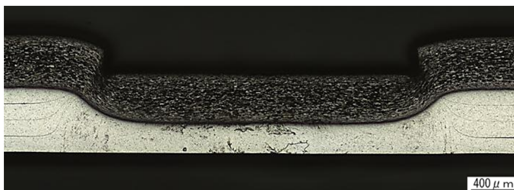
Fig. 4-31 Micrograph showing cross section of multilayered joint
