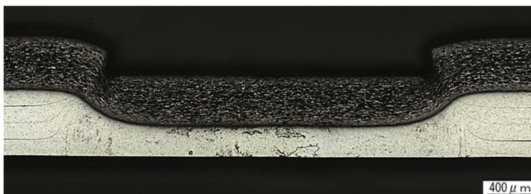
Fig. 4-31 Micrograph showing cross section of multilayered joint
