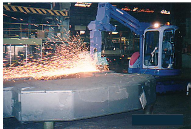
(b) Grinding in large machine factory
