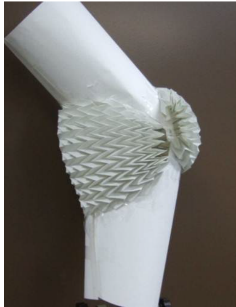
Figure 2.9. Single axis joint with curved shell folding structures [41].
