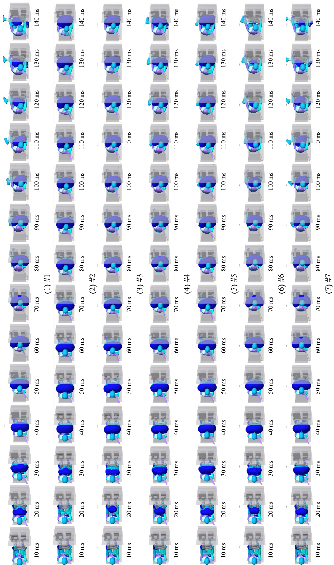
Fig. 5.12(a)(i) Top view of occupant behavior (crash pulse and cabin-deformation as mechanical loads at \Delta V of 20 m/s)
