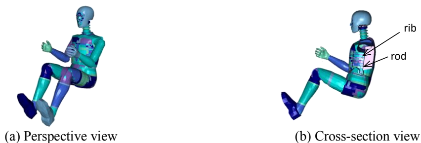
Fig. 2.10 Occupant model (Hybrid III 50 th percentile dummy)
