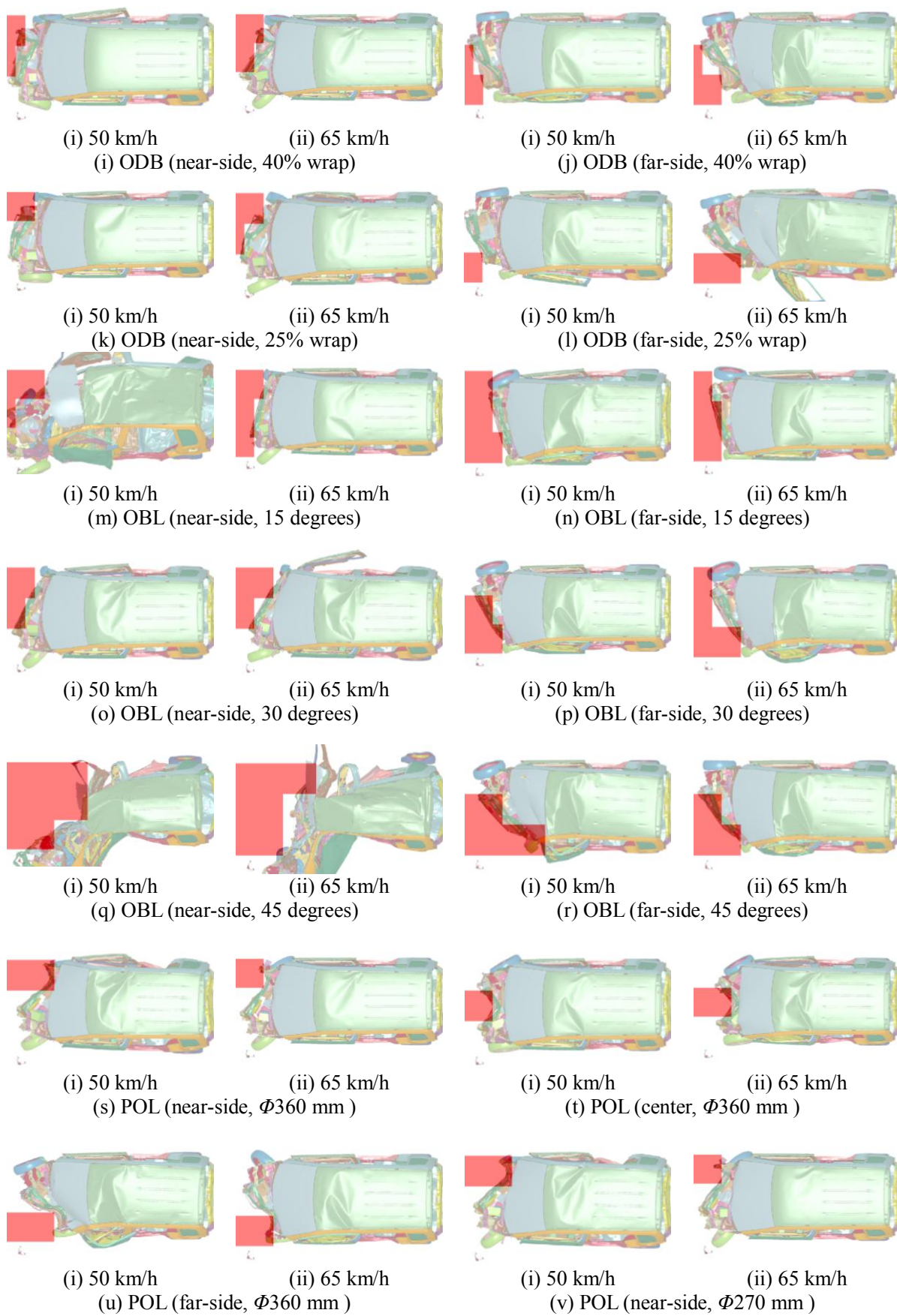
Fig. 3.4 Vehicle damage from top view in each crash pattern at the two level of V_0
