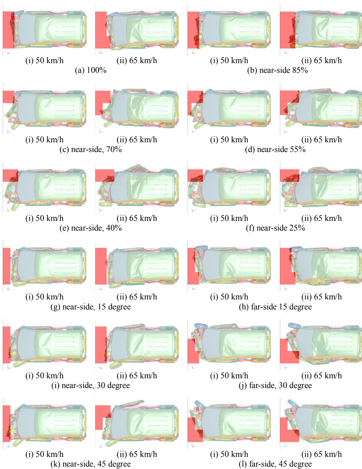
Fig. 3.11 Vehicle damage from top view in each crash pattern of VTV simulations at the two level of V_0
