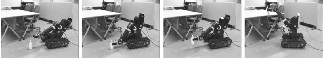
Fig. 8.13: Carrying bottle while keeping posture of end-effector
