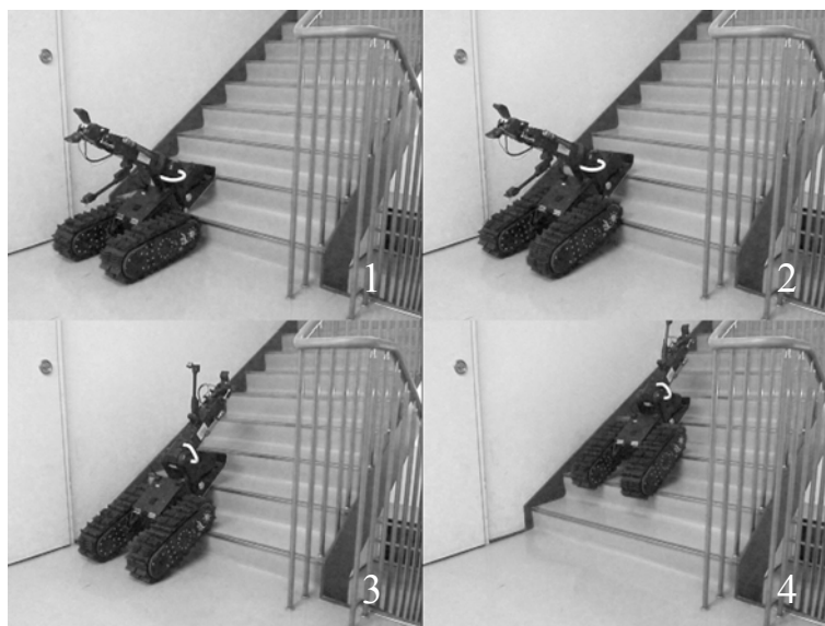
Fig. 8.6: Stairs climbing with sled
