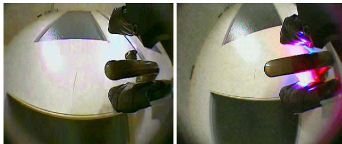
Fig. 7.17: Gripper camera view without LED(left), with LED(right)
