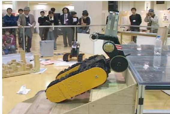
Fig. 2.8: HELIOS VIII- stairs climbing test
