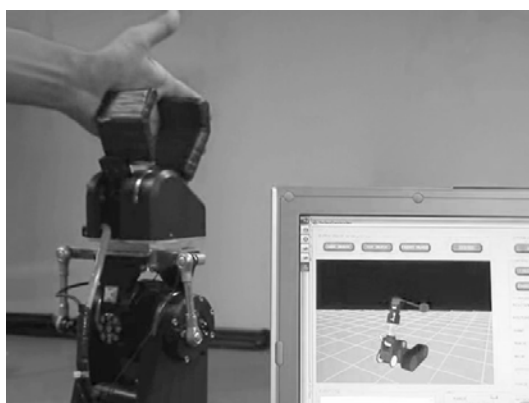
Fig. 4.11: Force vector displayed in GUI
