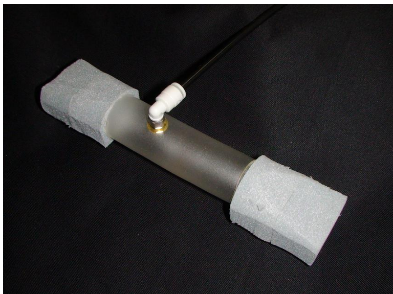
Fig. 4-15 An actuator bag with neoprene sponge
