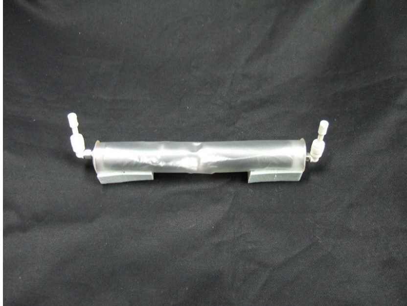
Fig.4-18 An actuator bag including neoprene sponge
