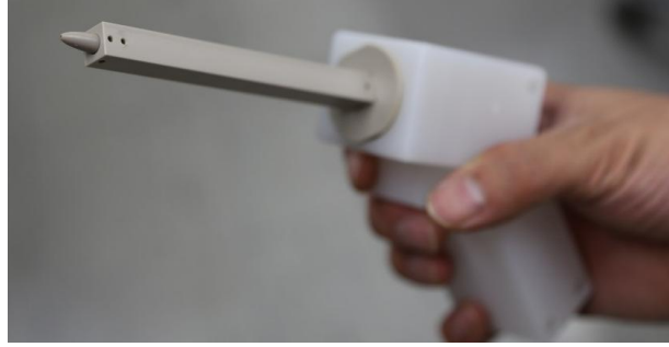
Figure 3. Apparatus of the nozzle for steam-jet application
