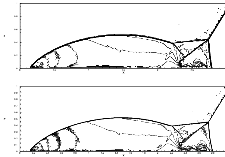
FIGURE 3.17: Numerical results of double Mach reflection at t = 0.2 with 120 \times 384 cells (top), 250 \times 800 cells (bottom).
