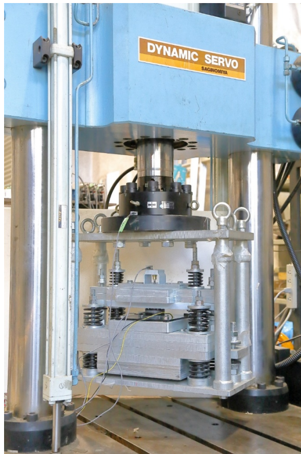
Figure 4.8 Setup of TMG on an excitation machine
