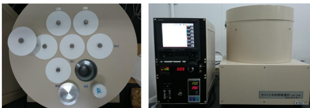
Fig. 1-2-1 Outer mixing type conduction calorimeter (Six-point type)
