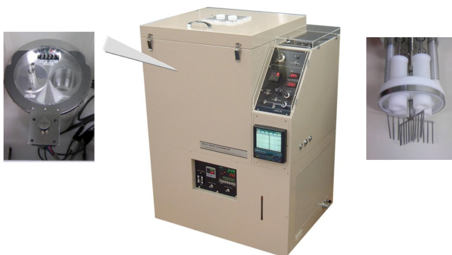
Fig. 1-2-2 Inner mixing type conduction calorimeter
