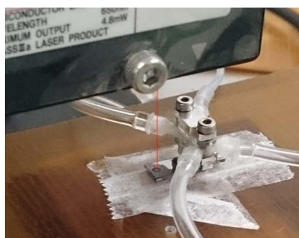
Fig. 5.42 Measurement of deflection of micro-diaphragm by laser displacement meter
