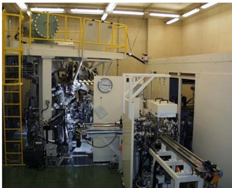
Fig. 3-5. Combined Space Effects Test Facility.
