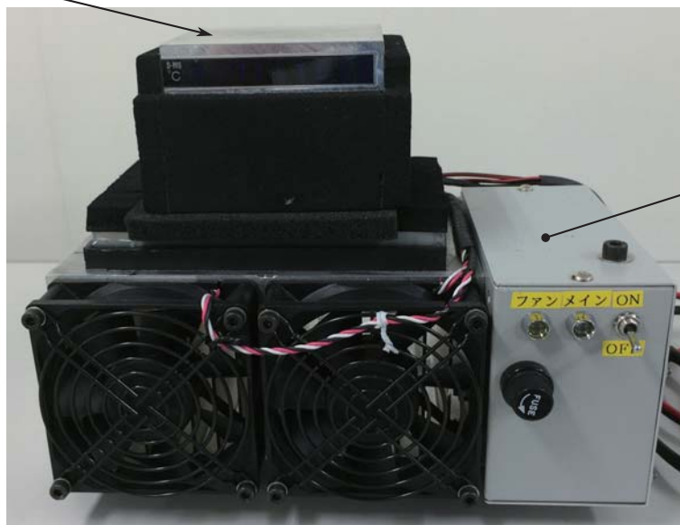
Fig. 2.10: Outline view of the refrigeration equipment. The refrigeration equipment is placed underneath of the metal block. The size of metal block is 70 mm long, 80 mm wide and 60 mm high.
