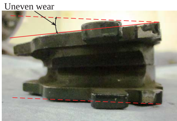
Fig. 1.3: Picture of unevenly worn pads.
